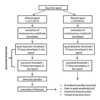
Fig. 1. Flow diagram of the applied procedure.
